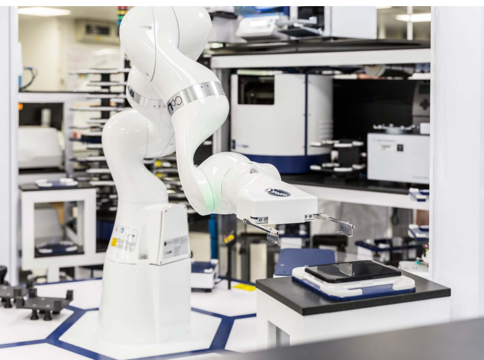
NiCoLa-B is an advanced drug discovery robot that can test up to 300,000 compounds a day, working three times more quickly than previous drug discovery robots. The MRC has provided funding for academic researchers to run high throughput drug screening projects within the AstraZeneca UK Centre for Lead Discovery. Image courtesy of AstraZeneca©
